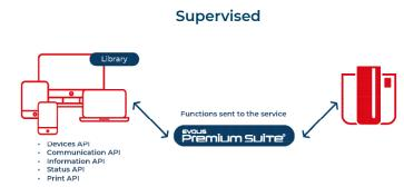
Using supervised mode of communication with the printer allows to delegate printer supervision and error management to the Evolis Premium Suite 2\* service. This option simplifies the printer integration since all errors during printing are automatically handled by Evolis Premium Suite 2\* by displaying notifications and allowing the user to solve the problem.
