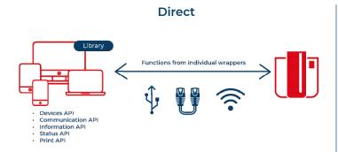
Direct mode of communication with the printer allows developers to manage by themselves the printer supervision and error management into their application. This option offers more flexibility and customization to answer specific needs regarding Evolis printer's integration.
