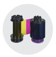
The Evolis YMCKI ribbon is specific to retransfer technology. The inhibitor special coated panel (I) prevents the design from being printed on specific parts of the cards such as magnetic stripes, chips and signature panels.
