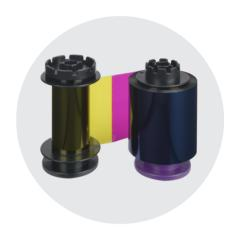
The Evolis YMCKH ribbon has been designed to enable Evolis retransfer printers to use various card substrates other than PVC: Polycarbonate (PC), PET-G and ABS. The Heat Seal (H) panel is a special coating that is applied after the Y, M, C, K panels to enable the good transfer of the printing on the card with uneven surface.
